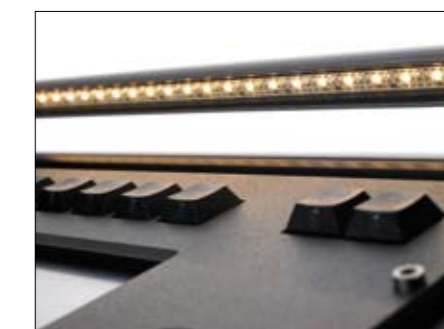
LEDs light up the programmable view keys
