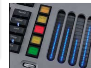
The fader belts give you immediate visual feedback of parameters
